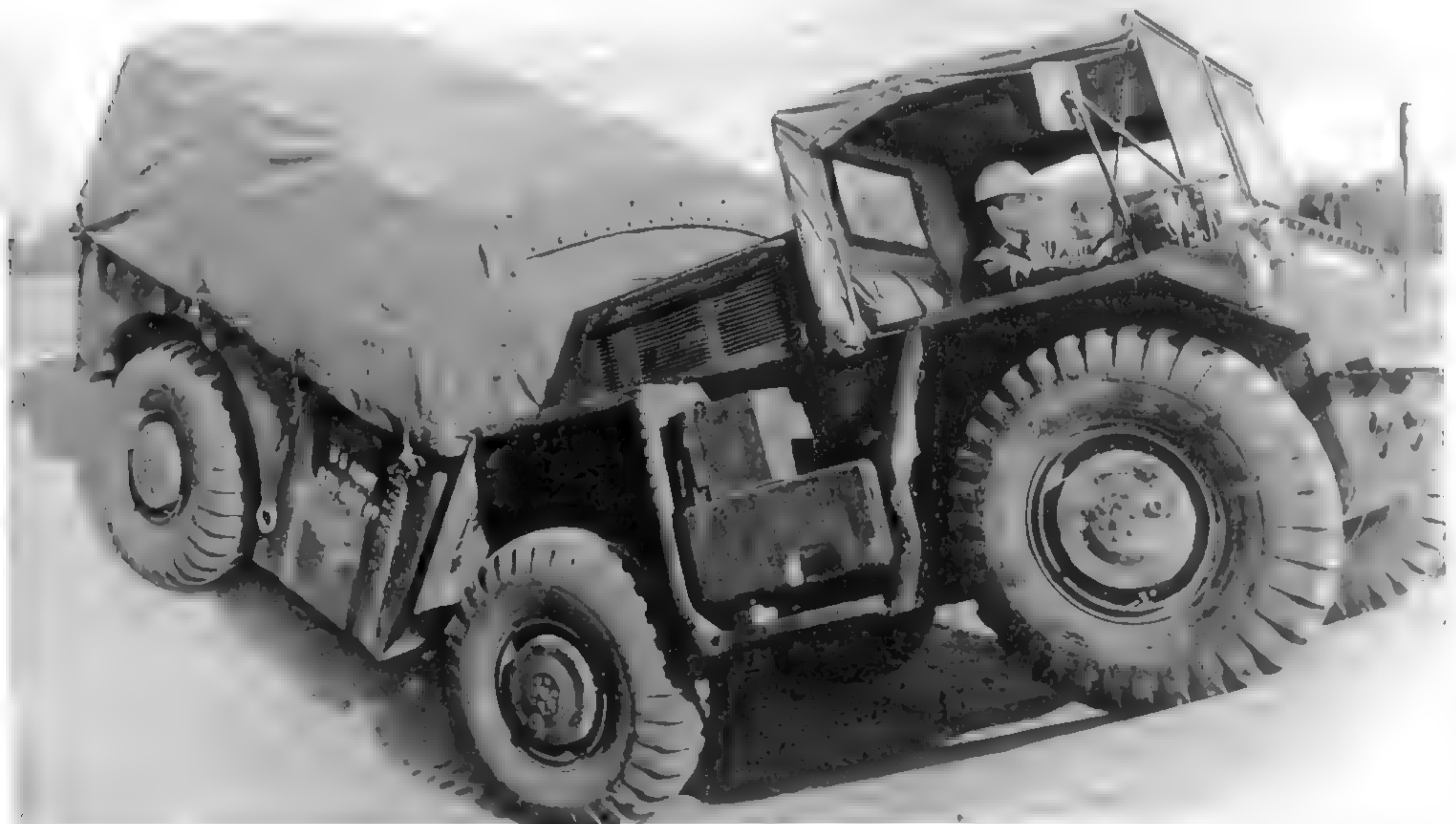
The sloping rear fenders and sloping engine compartment provided extreme flexibility, and kept the Gama Goat's tires in contact with the ground. (U.S. Army photo)
